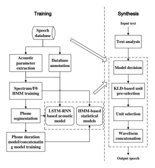
Figure 1: Flowchart of the IFLYTEK unit selection system.
